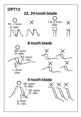
the blade is fed faster than its cutting capability.
